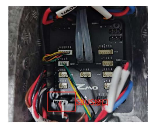
SBUS connection wire, use the connection wire that comes with SIYI to connect to the flight control SBUS interface,
